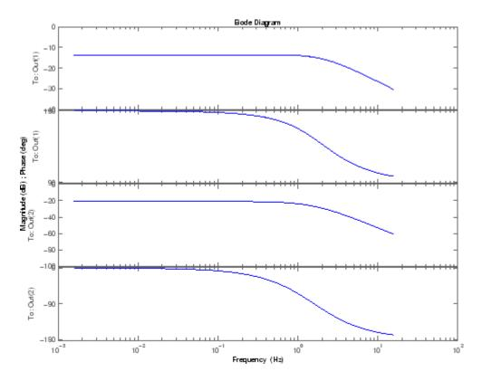
Just as with the umat and uss classes, the Uncertainty property is a structure containing the uncertain elements. Direct access to the elements is facilitated through Uncertainty. Change the nominal value of the uncertain element named 'p1' within sysg to 14, and replot the Bode plot of the (new) nominal system.
