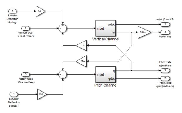
**3** Specify uncertain variables for the gain blocks Zd and Mw in the Aircraft Dynamics Model subsystem.
