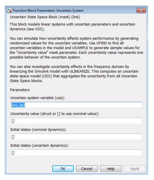
The Uncertain System block uses the uncertain system variable unc\_sys. This variable is defined in the Model workspace as unc\_sys= ss(ureal('a',-1,'Range',[-2 -.5]),1,5,0)\*(1+0.1\*input\_unc). The
