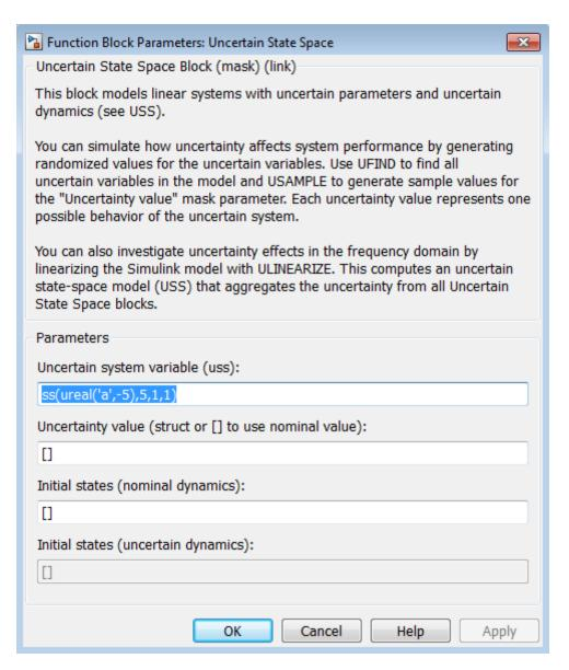
3 Specify an uncertain state-space model in the **Uncertain system variable** (uss) field. The model must be an uss object or any other model that can be converted to uss, such as umat, ureal and ultidyn. The model depends
