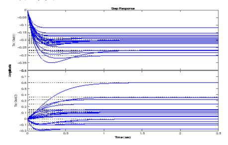
The command step can be called directly on a uss object. The default behavior samples the uss object at 20 instances, and plots the step responses of these 20 models, as well as the nominal value.
