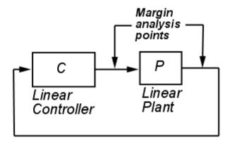
Analyzing stability margin of Simulink models differs from analyzing stability margin of LTI models because you can enter specific margin analysis points in the Simulink model. For more information on how to assign margin analysis points in Simulink models, see the "Usage with Simulink" section of the loopmargin reference page.
